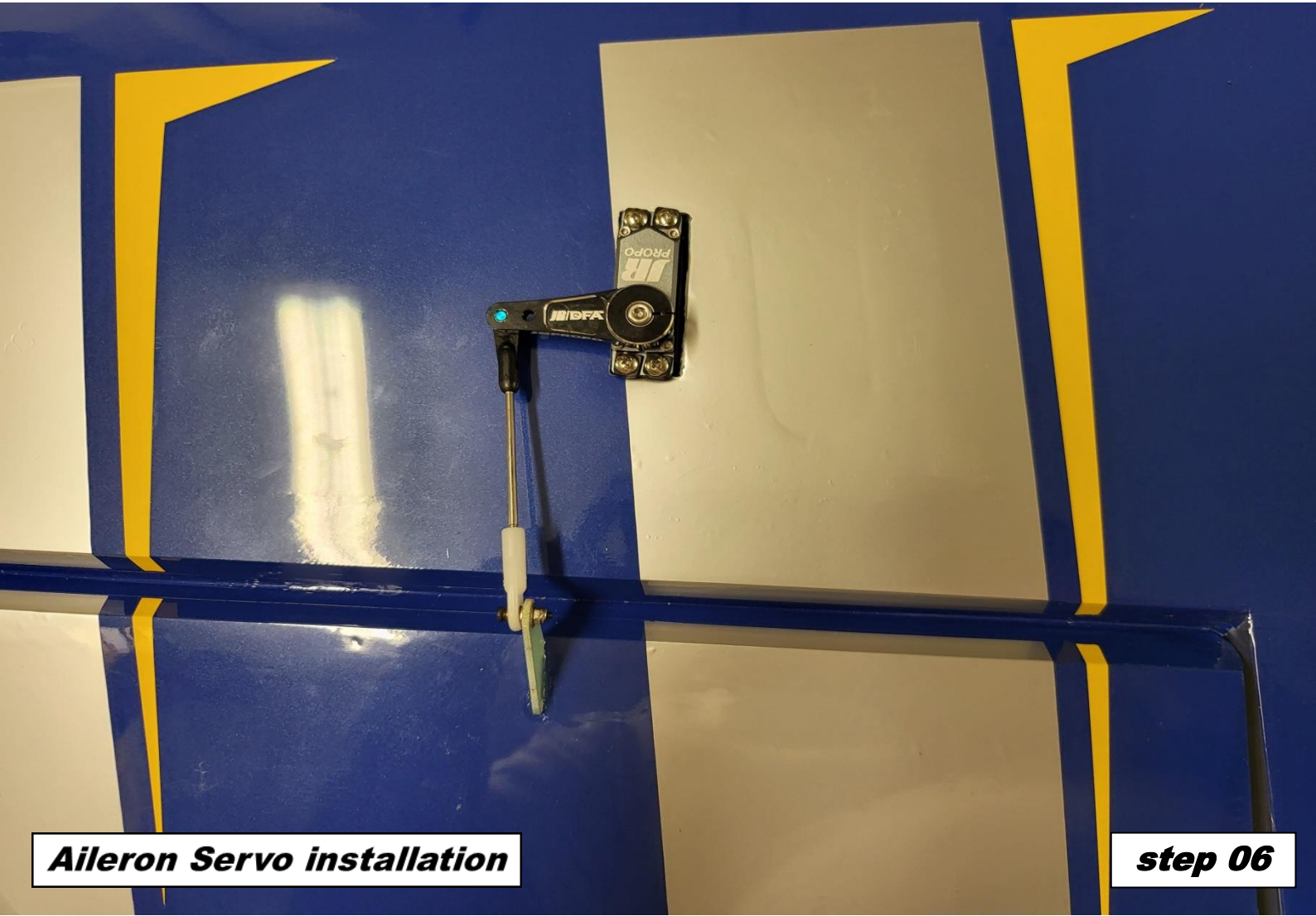
Aileron Servo installation
